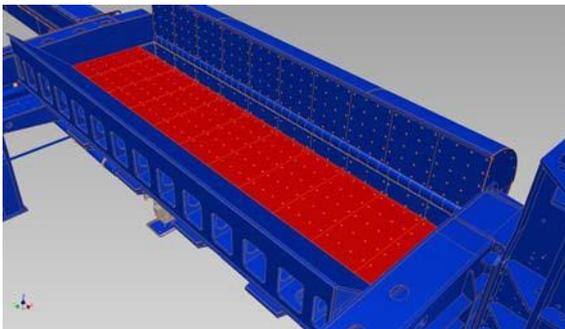
The shear lets you work in parallel or angular mode. With the powerful side compression block in the parallel position and the compression lid half closed, the scrap in the box is compressed as far as possible.
