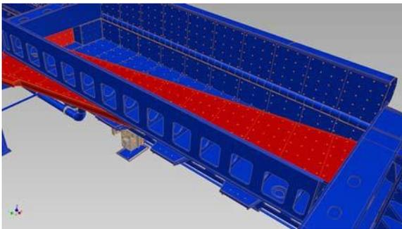
By selecting the angle adjustable mode the full compression force is exerted at one end of the piece of scrap providing immense crushing power.
